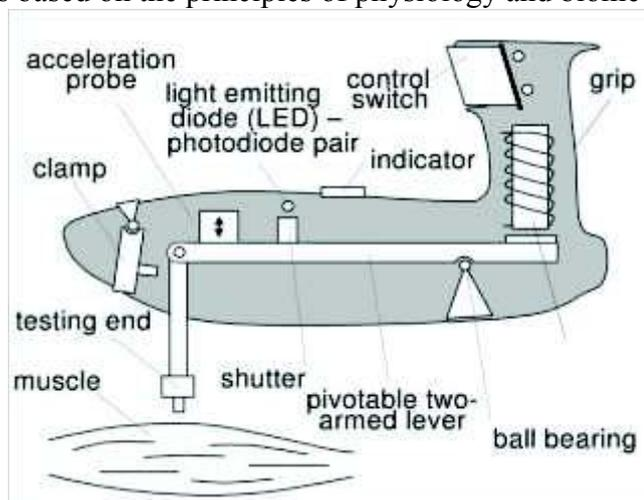
**Figure 1.** Myotonometric measure device MYOTON-3 (Myoton, 2010).
